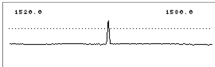
PRBS modulation graph showing raised noise floor.
